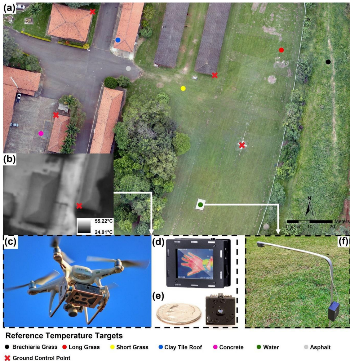
Figure 1. Data acquisition scheme for aerial analysis. (a) Distribution and types of reference targets and ground control points; (b) Thermal image snapshot; (c) UAV platform with the Lepton camera onboard; (d) Lepton camera; (e) FLIR Lepton 3.5 OEM sensor; (f) Ground reference temperature platform with the MLX90614 sensor.
